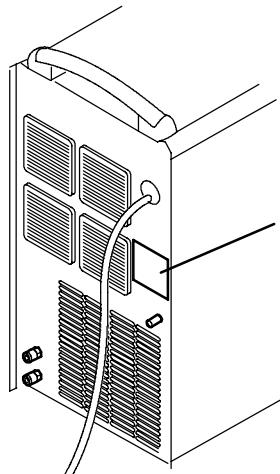
Check that the unit is connected to the correct mains power supply voltage, and that it is protected by the correct fuse sizes. A protective earth connection must be made, in accordance with regulations.
